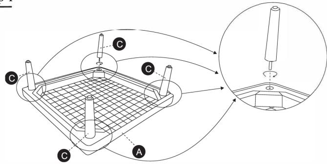
Turn Seat Frame (A) upside down on a clean, non-marring surface. Align bolts on Legs (C) with receiving holes in Seat Frame (A), as shown. Rotate Legs (C) clockwise until snug. DO NOT over tighten.
